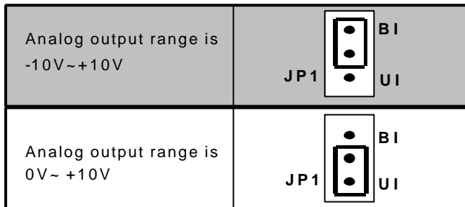
Figure 2.2 Analog output range setting
